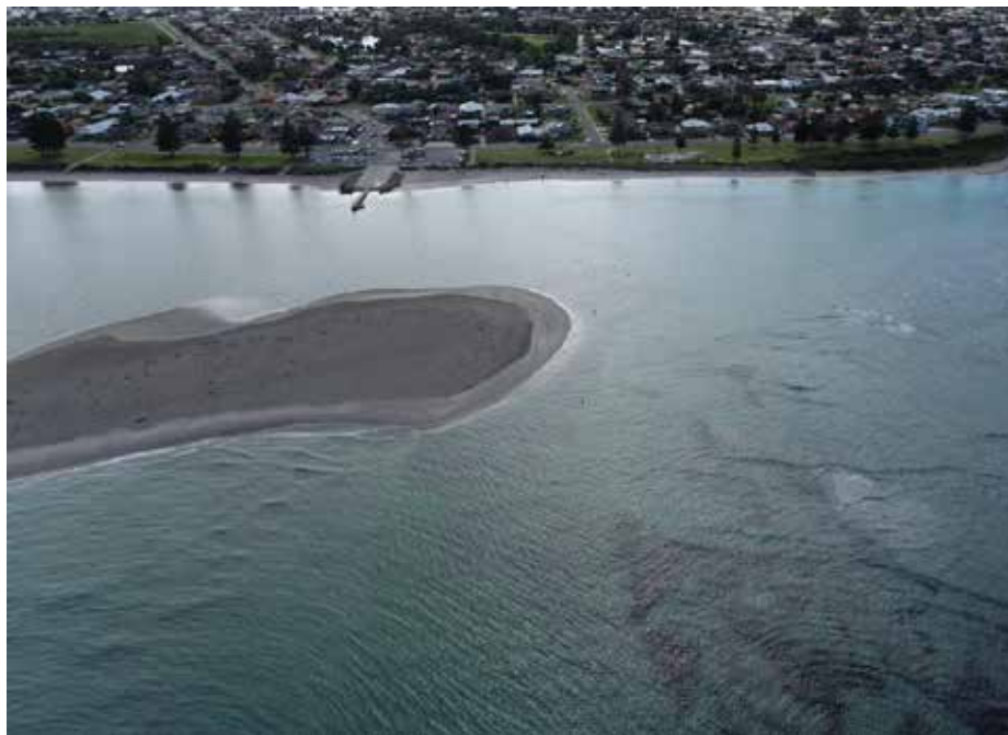
Tern Bank Sandbar sediment migration into Bent Street Navigation Channel – August 2022
