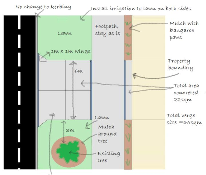
Build a crossover, exposed aggregate finish and keep existing mountable kerbing
