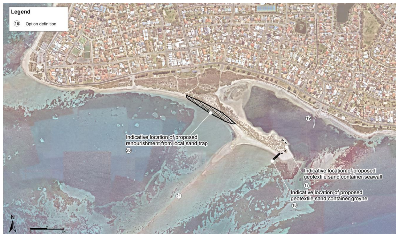
Figure 8-2 Sector 5: Option 2 – Stabilise Tern Bank with terminal groyne and sand trap management (local)
