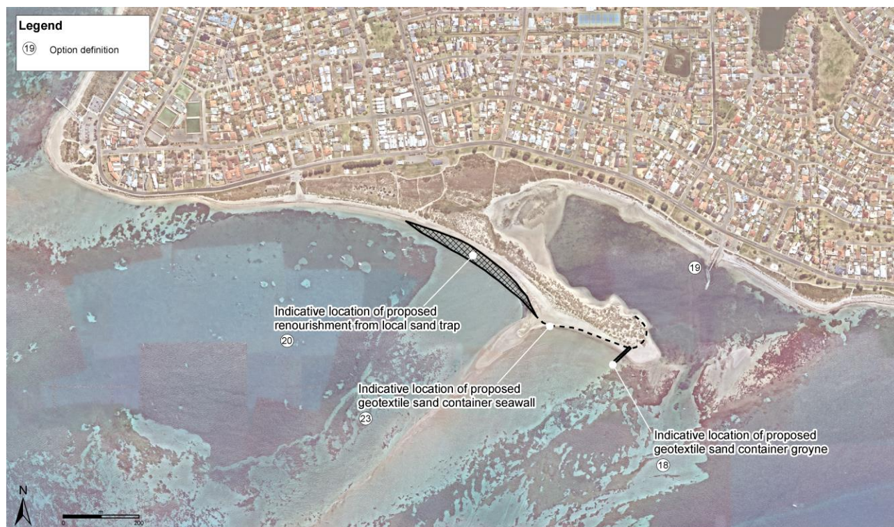
Figure 8-3 Sector 5: Option 3 – Stabilise Tern Bank with seawall and terminal groyne and sand management (local)
