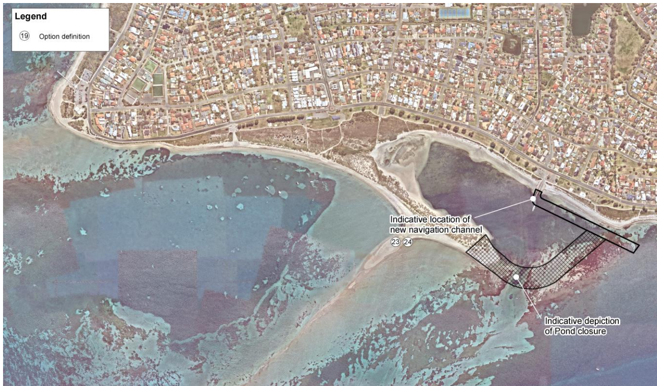
Figure 8-4 Sector 5: Option 4 – Tern Bank natural progression with realigned channel parallel to coast nearshore
