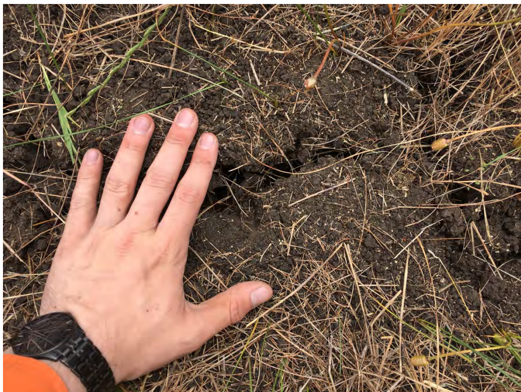
Photograph 3: Shrinkage cracks in Organic Clay material in east of site
