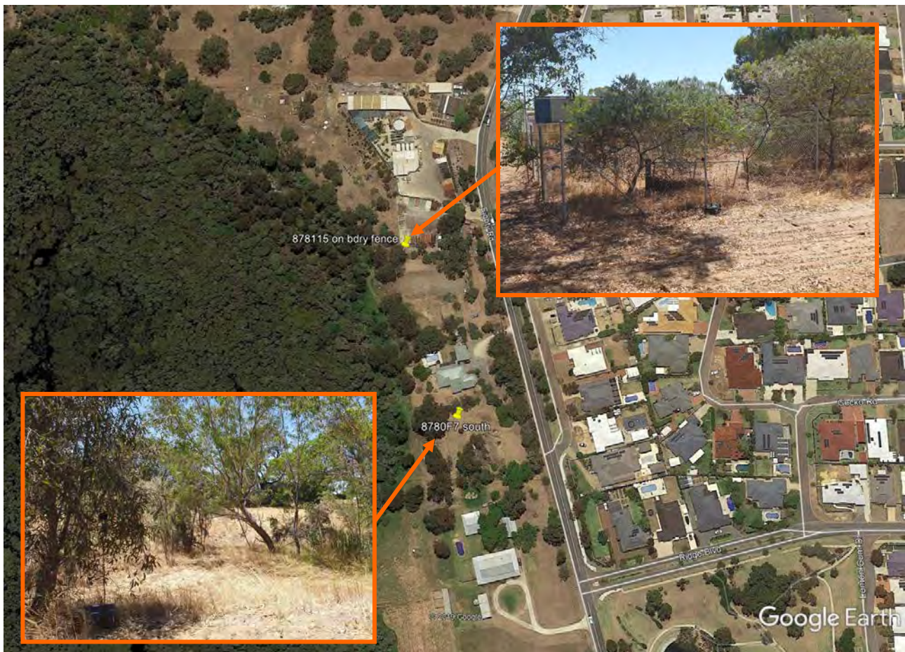
Figure 1: Locations of Noise Data Loggers on Site
