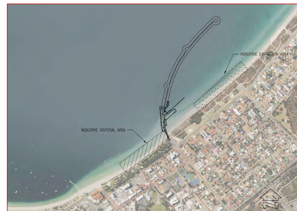
Figure 6: Indicative sand bypassing operation
