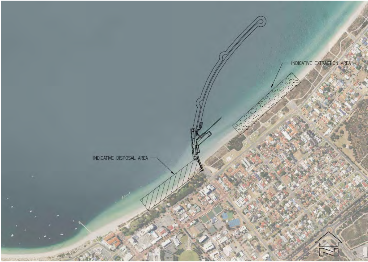
Figure 4.3 Indicative Sand Bypassing Operation
