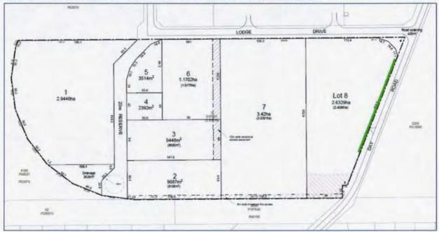
Figure 3-3 Potential Crossover Locations for Lot 8 (Assuming 60km/h Frontage Road Speed)
