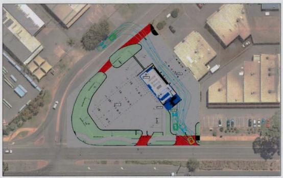
115 Dixon Road, East Rockingham Austroads 2013: 12.5m SU Truck Service Truck Entry Vehicle Body Wheel Path 500mm Clearance
