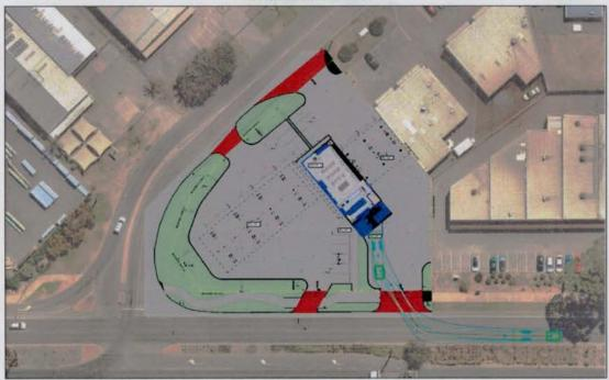
115 Dixon Road, East Rockingham Austroads 2013: 12.5m SU Truck Service Truck Exit LEGEND Vehicle Body Wheel Path 500mm Clearance
