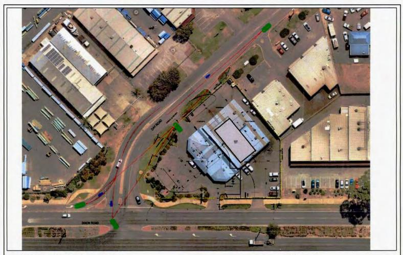
115 Dixon Road, East Rockingham Sight Distance Assessment Speed = 60km/h Minimum SSD = 65m t20.134.sk11 14/07/2020 Scale: 1:500 @ A3
