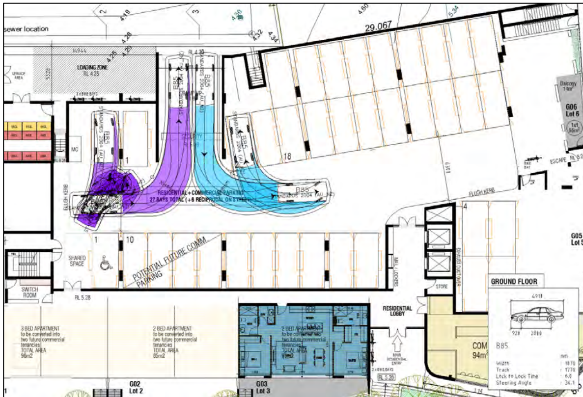
Figure 5-3 Swept Path - B85 Passenger Vehicle
