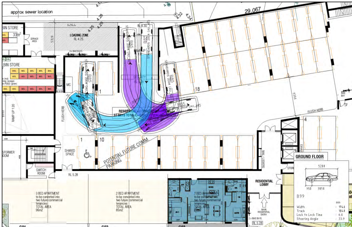
Figure 5-5 Swept Path – B99 Passenger Vehicle
