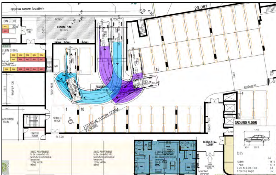
Figure 5-2 Swept Path - B85 Passenger Vehicle
