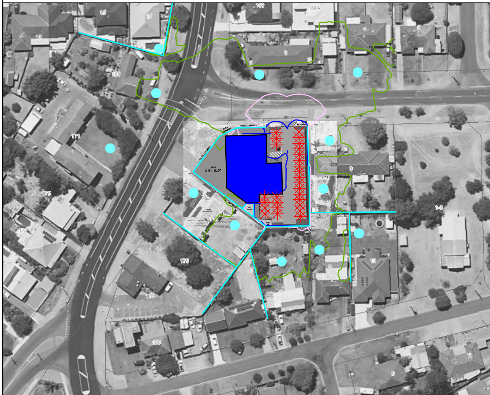
Figure 4-3 Car Door Closing Noise Contour Plot (1.4m AGL), dB L_{AMAX}
