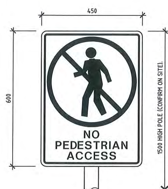
S9 S02 CAR PARK SIGNAGE NON-ILLUMINATED ALUMINIUM REFLECTIVE SIGN ON GALVANISED STEEL POLE TYPICAL.
