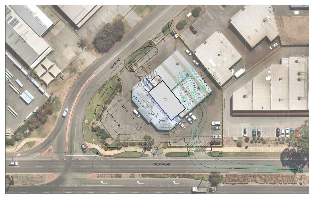
115 Dixon Road, East Rockingham Austroads 2013: 19.0m Semi-Trailer Truck Exit onto Dixon Road from 2nd Bowser LEGEND Vehicle Body Wheel Path 500mm Clearance
