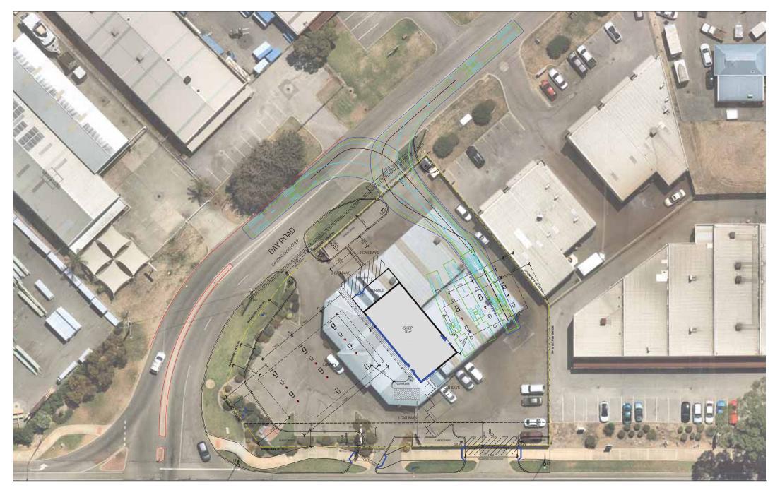
115 Dixon Road, East Rockingham Austroads 2013: 19.0m Semi-Trailer Truck Left-in & Right-in Entries to 3rd Bowser LEGEND Vehicle Body Wheel Path 500mm Clearance
