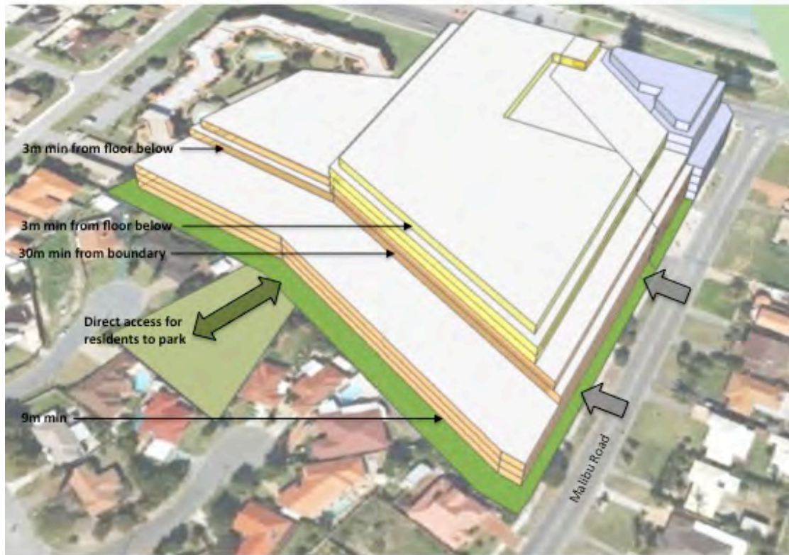
Maximum allowable building envelope - View from North
