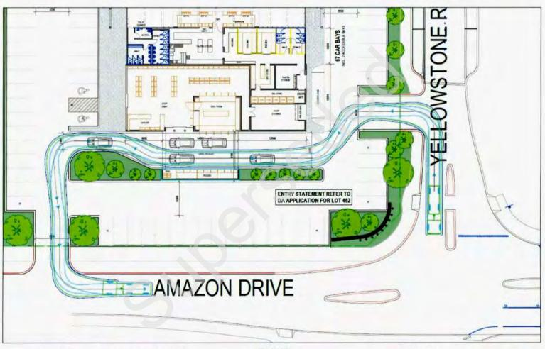
Proposed Tavern, Amazon Drive, Baldivis Passenger Vehicle with Trailer Vehicle with trailer circulation
