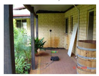
Figure 3.1 – Automatic Noise Data Logger
