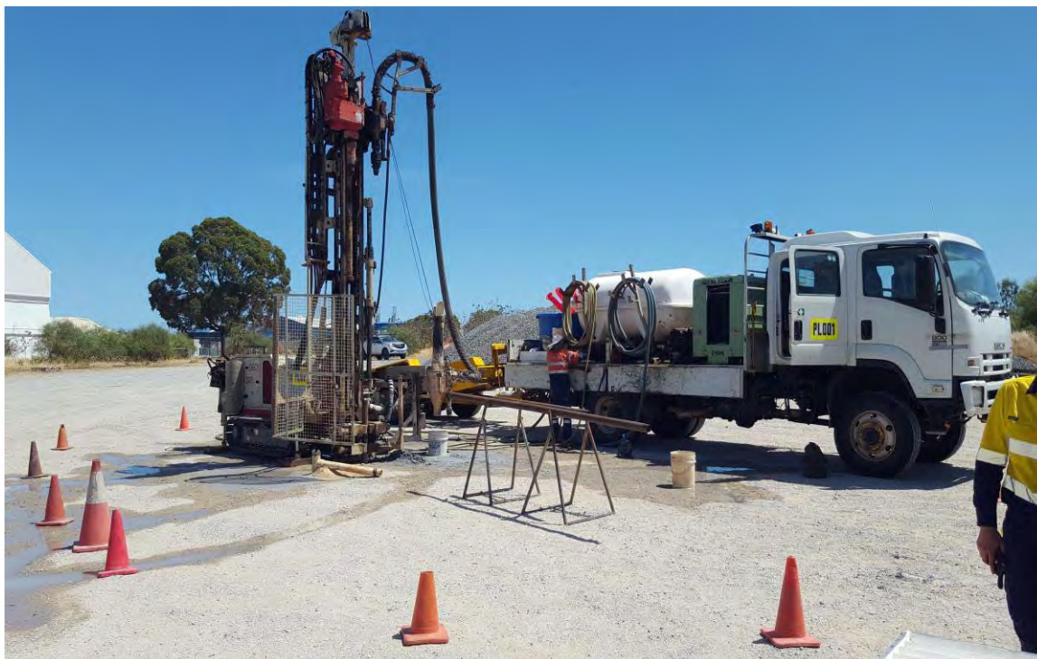
Photograph 7: Typical air core drill rig setup
