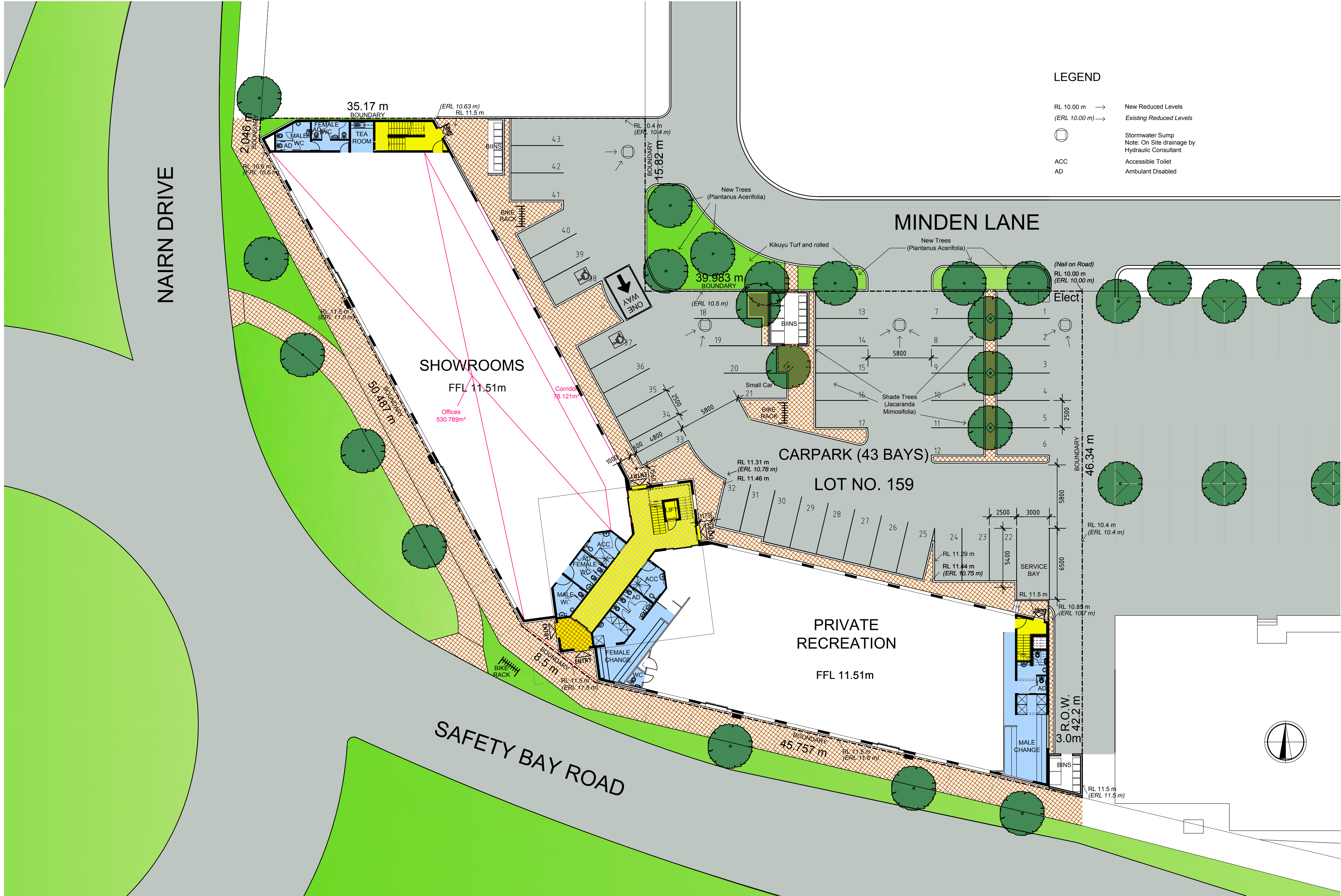
SITE & GROUND FLOOR PLAN 1:200
