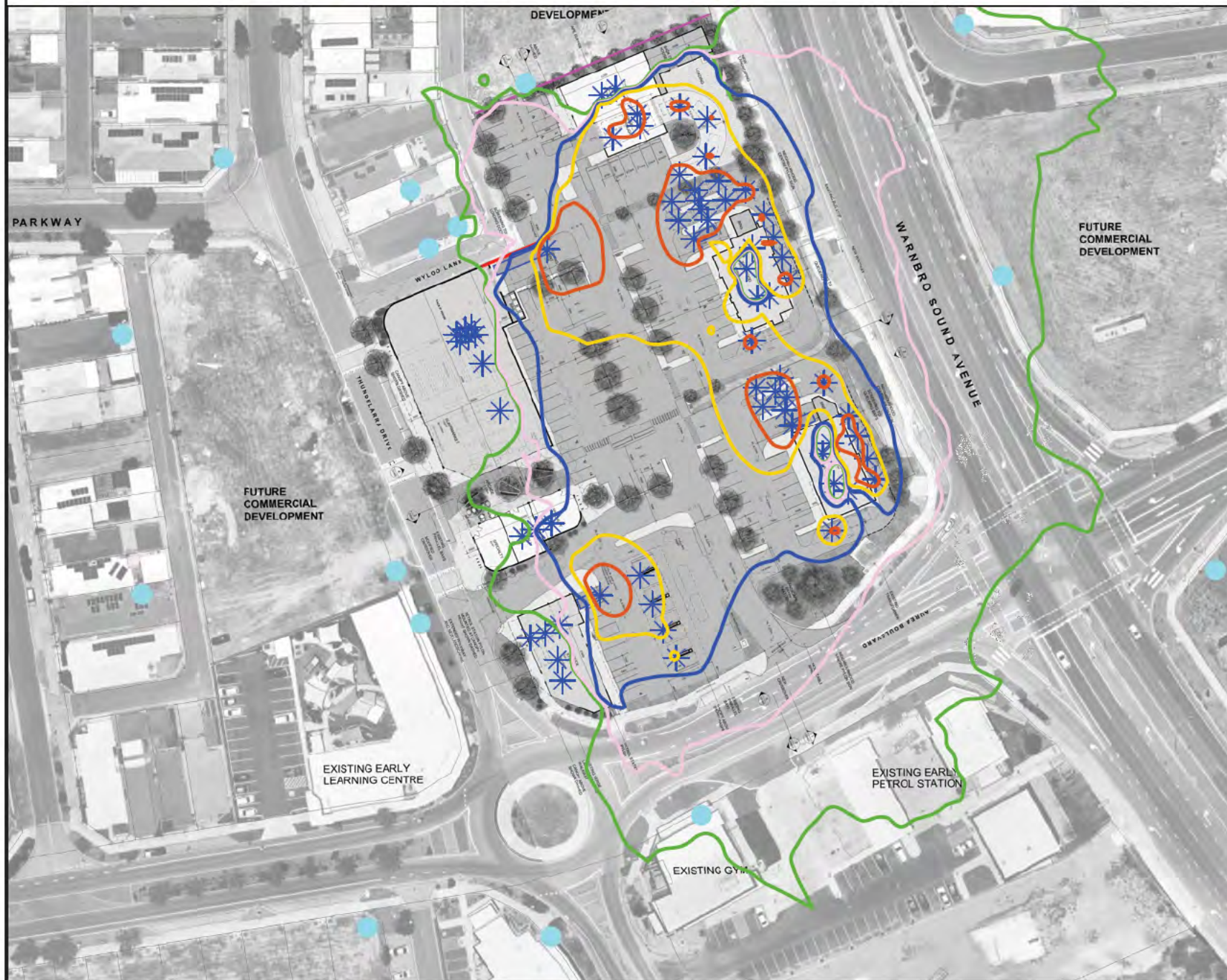
Figure 4-2 Scenario 2 Noise Ground Floor, dB L A1
