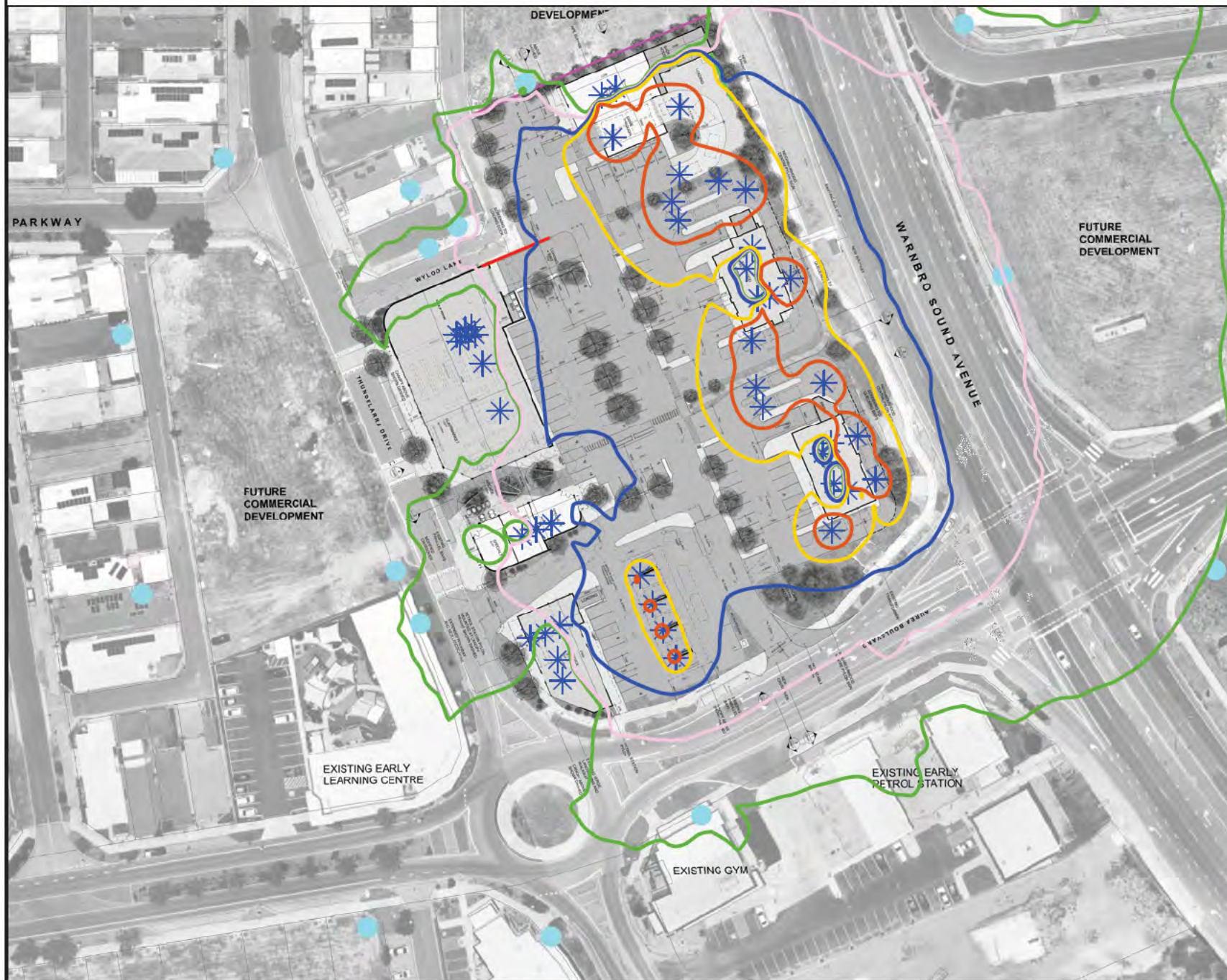
Figure 4-1 Scenario 1 Noise Ground Floor, dB L_{A10}
