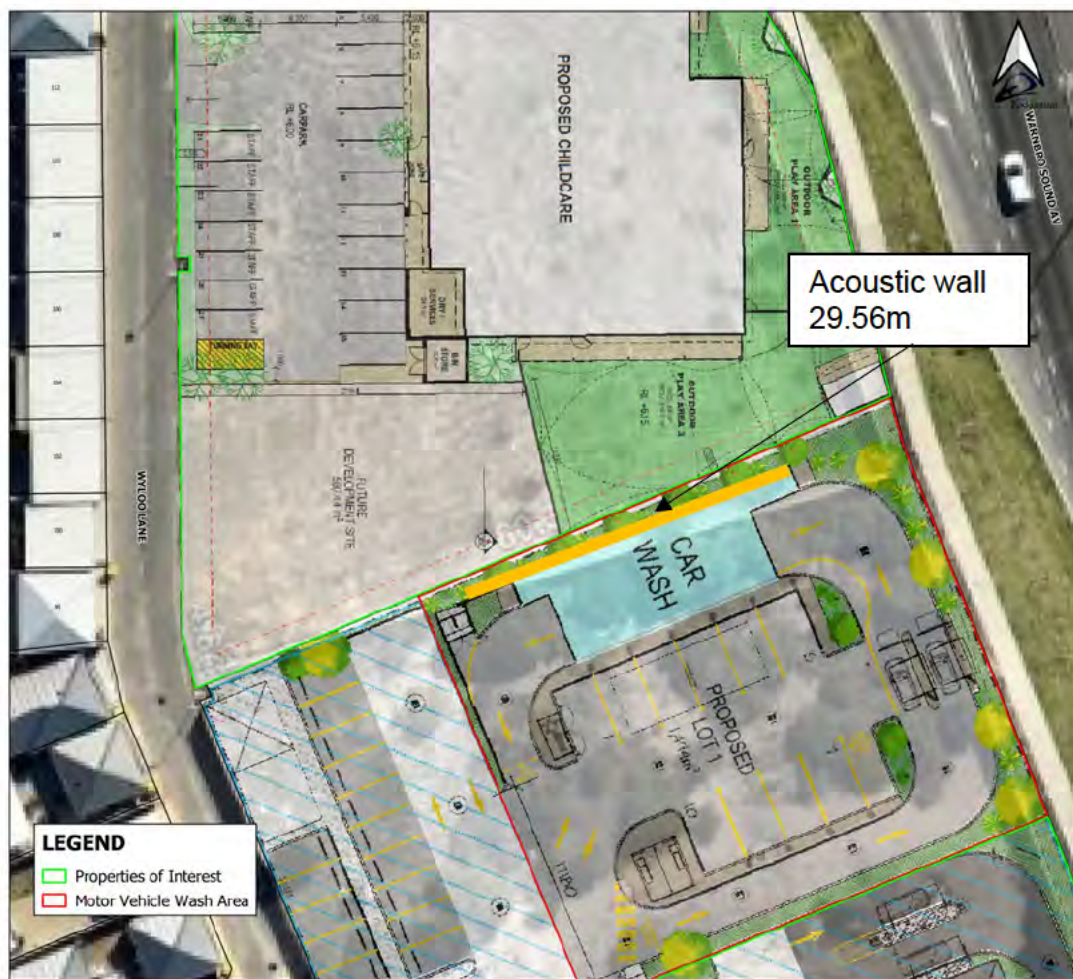
Figure 6. Extent of Acoustic Wall to Northern aspect
