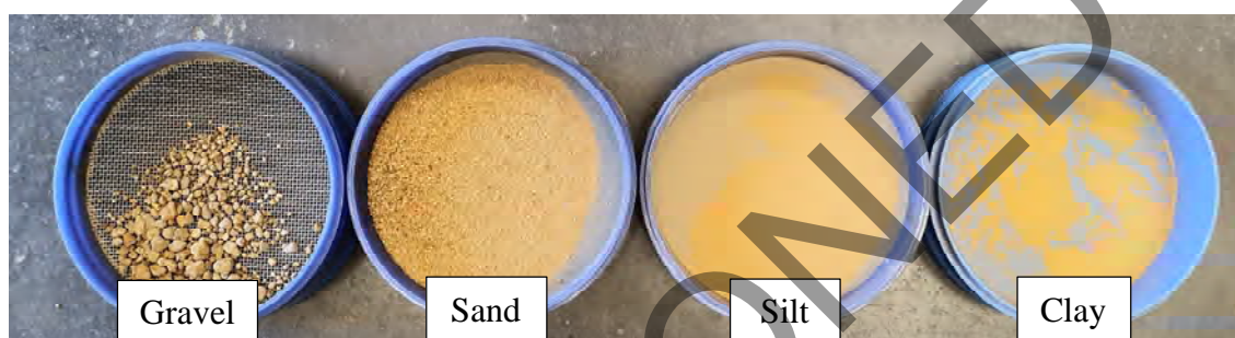
Figure 4.13 Soil fractions of sample TP2.
