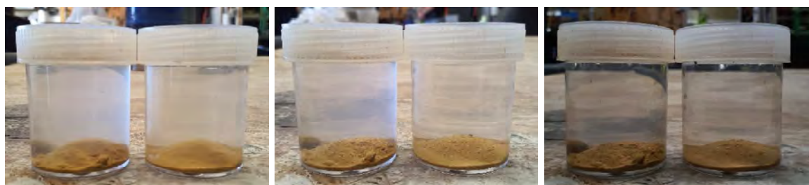
Figure 4.10 Dispersion and gypsum responsiveness TP2. In each photo the RHS jar is soil in gypsum solution. LHS jar is soil in water. (L set) after 15 minutes, (M) after 2 hours, (R set) after 20 hours.
