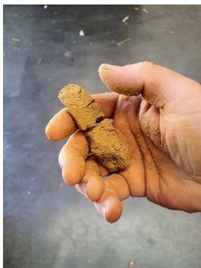
Figure 4.12 (L) Ribbon test. (R) Permeability TP2.
