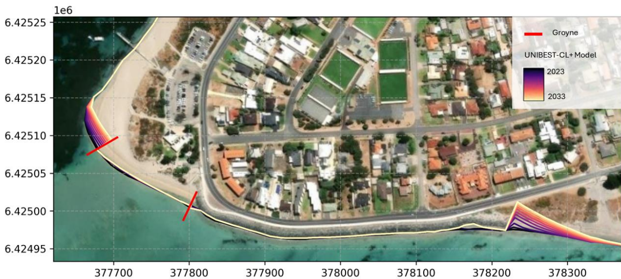
Fig. B.3.4-5: Shoreline modelling results, modelled with two groynes (red line) under a present day shoreline (2023).
