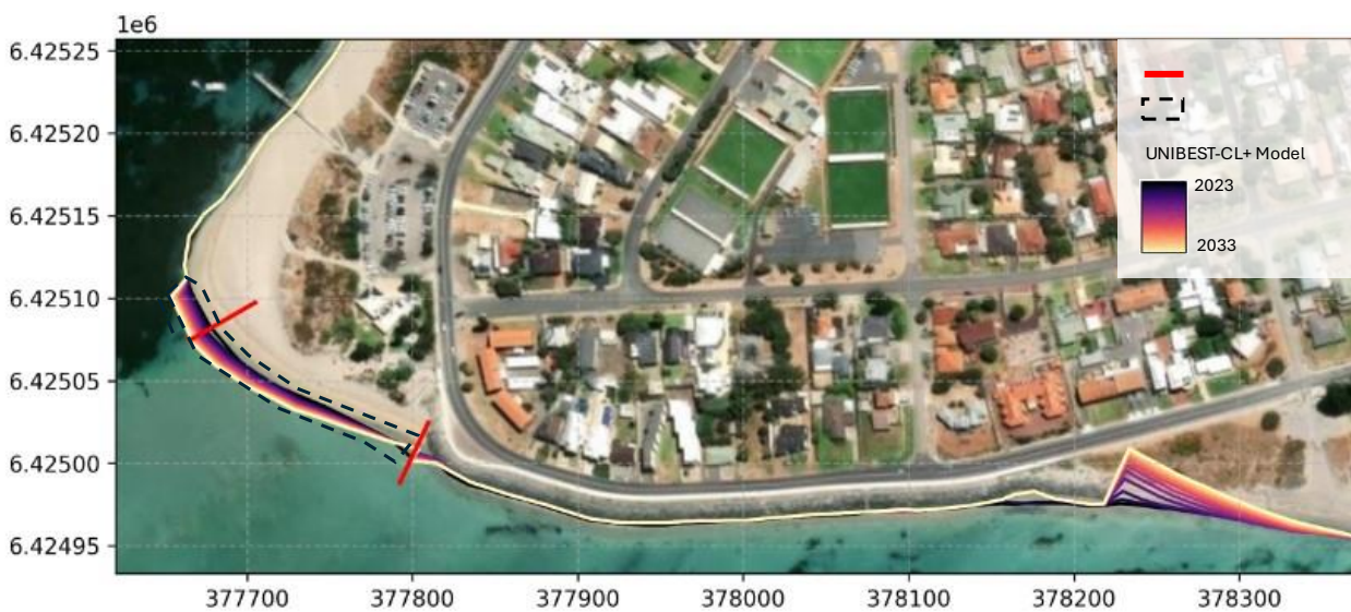
Fig. B.3.4-7: Shoreline modelling results, modelled with beach nourishment (black dotted line) between the two groynes (red line) and a present-day shoreline (2023)
