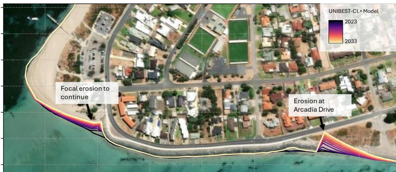
Figure 5-3: Coastline modelling results, adopting a 'Do Nothing' approach, modelled with average yearly conditions. NB: average conditions underestimating rate of erosion at west tip of revetment.
