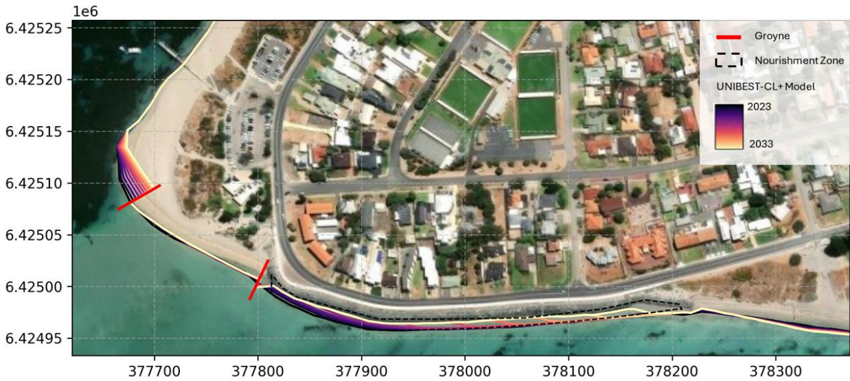
Fig. B.3.4-6: Shoreline modelling results, modelled with two groynes (red lines) and sand nourishment at the toe of Arcadia Drive revetment (black dotted line).
