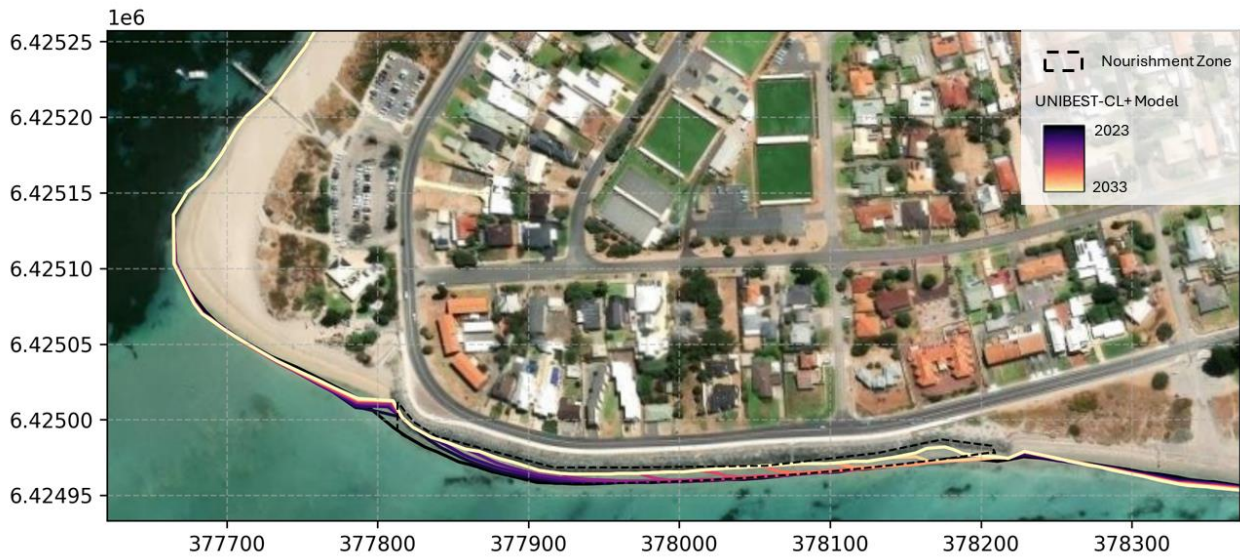
Fig. B.3.4-2: Shoreline modelling results, modelled with sand nourishment at the Arcadia Drive Revetment wall toe and beach nourishment at Mersey Point.
