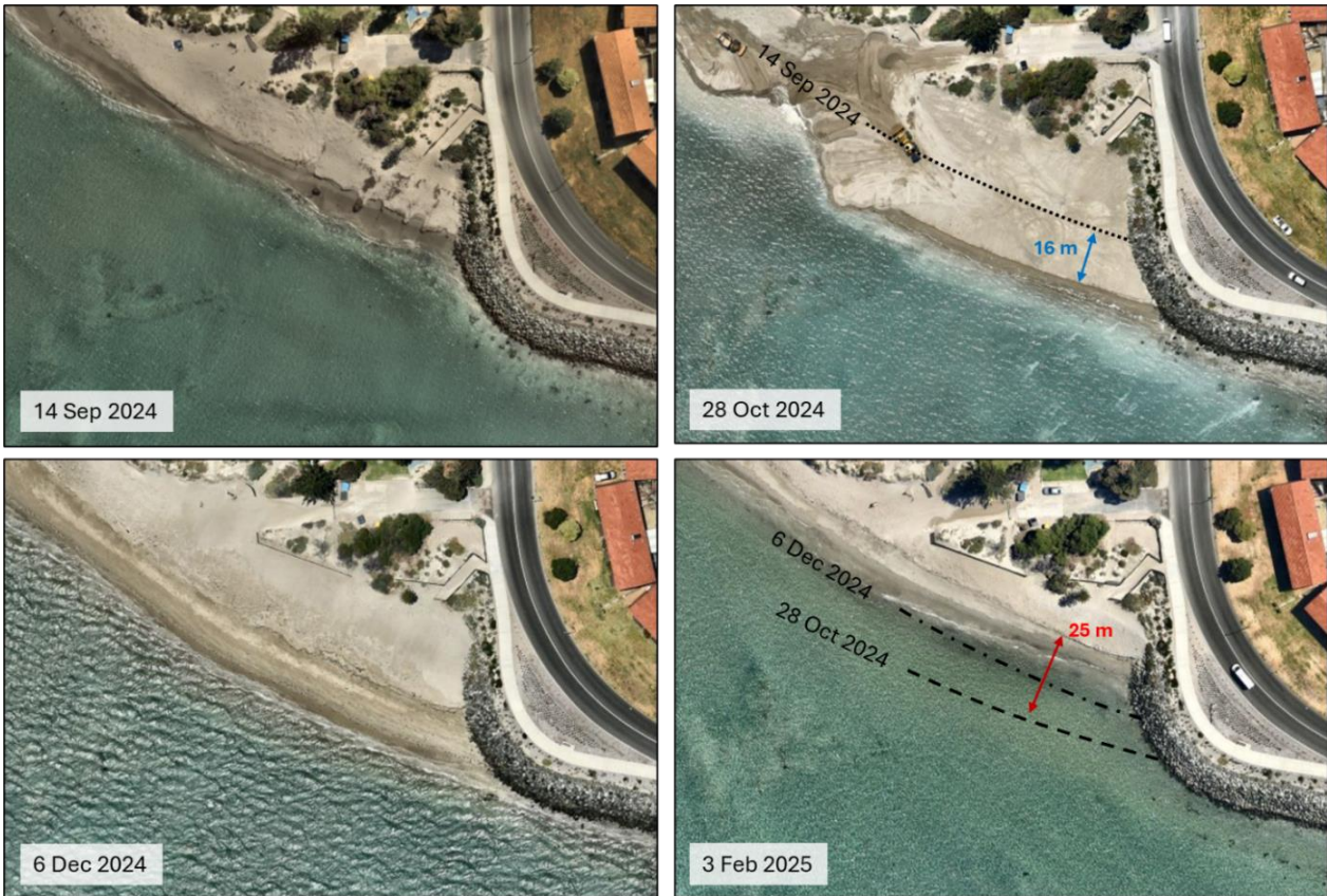
Figure 5-4: Aerial images from recent October 2024 back-passing campaign (Nearmap imagery) showing extent of focal erosion following nourishment.
