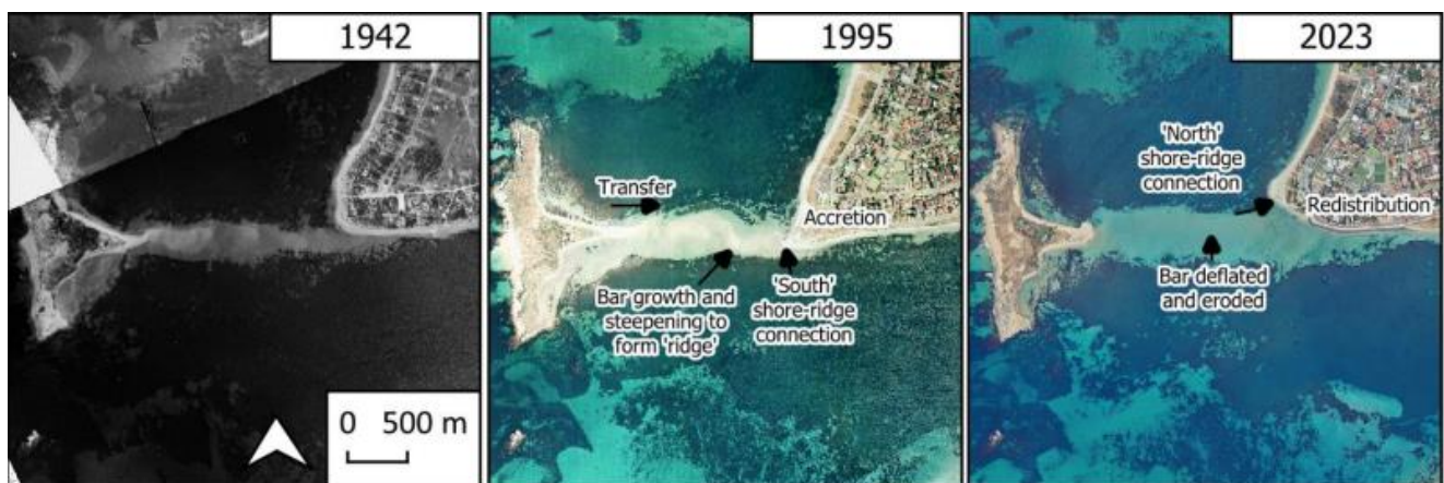
Figure 5-1: Penguin Island-Mersey Point sand bar evolution (Seashore Engineering, 2024).
