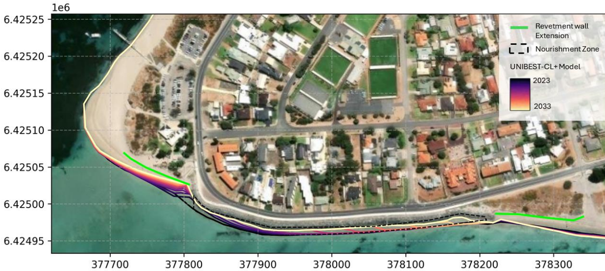
Fig. B.3.4-4: Shoreline modelling results, modelled with sand nourishment (black dotted line) at the toe of the Arcadia Drive revetment wall (green line), and the extension of the revetment wall.
