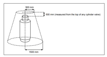
Figure 2: Minimum clearance to ignition sources.
