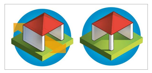
Examples of structures that have one open side, and 30% or more of the remaining wall area open and unobstructed.
