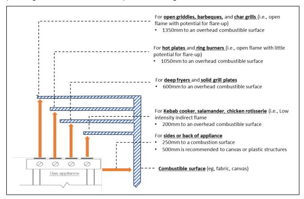
Figure 3: Appliance clearances from combustible material.
